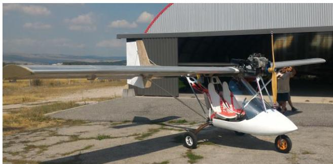
**Fuselage:** include - seats, belts, all controls, all factory welded parts, performed on CNC machines main beam, cockpit canopy with doors and rear section formed on mold – composite, nose wheel gear with nose wheel, main landing gear, 8 inch “heavy duty” alum wheels and mechanical disk brakes, polycarbonate windshield, wing struts, engine mounts for Hirth F23, fuel tank 20 l and all hardware.
